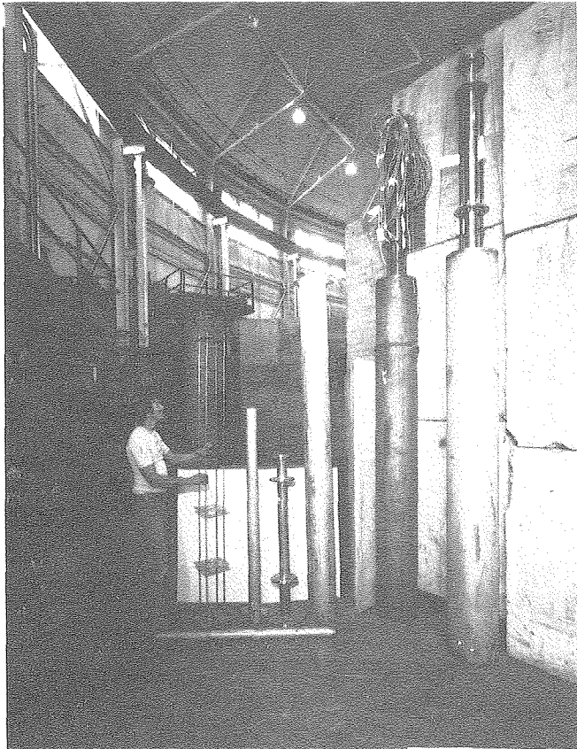
Figure 3. Photograph of full-scale heaters and components with test stand in the background. Heater at second from right is shown after running five weeks at 600°C.
