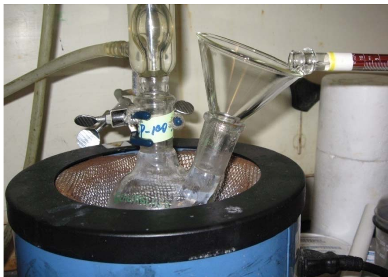
Figure A-2 Adding surface modifier
